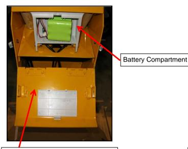
Rear Steel Cover opened and Plastic Internal Battery Cover removed.
