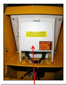
Plastic Internal Battery Cover visible after removal of Rear Steel Cover.
