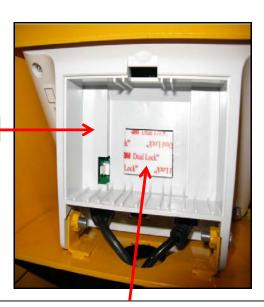
Battery removed revealing Velcro Pad. Tape should be removed from pad to expose stick surface. Battery Pack should be pressed against sticky surface.
